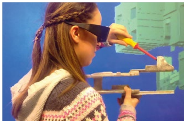
Fig.3 Mountability experiments – virtual assembly parts combined with real tools.
