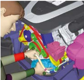
IC.IDO enables instant evaluation of flexible components, such as tubes and cables
